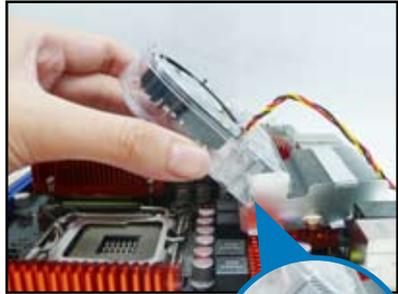
3. Carefully push down the fan until it snugly fits the heatsink, then connect the fan cable.
