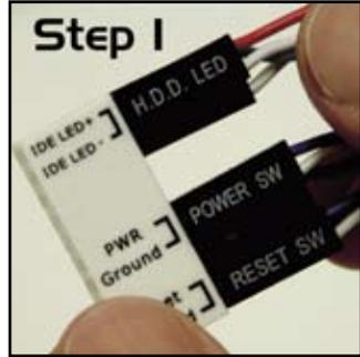
2. Install the ASUS Q-Connector to the system panel connector, making sure the orientation matches the labels on the motherboard.
