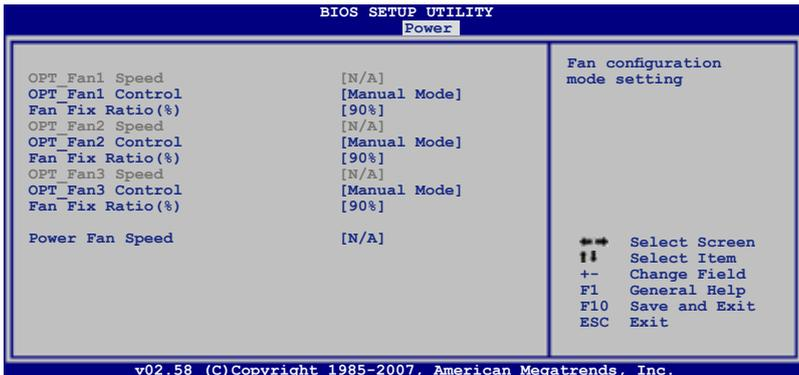
The onboard hardware monitor automatically detects the optional fan speed. If the fan is not connected to the motherboard, the field shows N/A.
