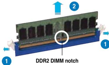
2. Remove the DIMM from the socket.
