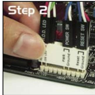
3. The front panel functions are now enabled. The figure shows the Q-Connector properly installed on the motherboard.
